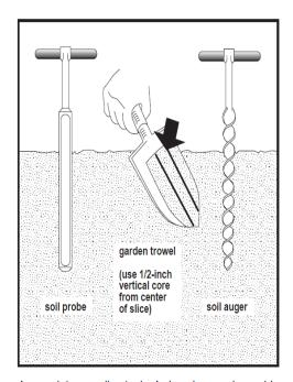
Appropriate sampling tools. A shovel or spade would also work, using the center core as witih the trowel.
